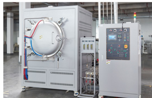
▲ 排胶炉 De-binder Furnace
